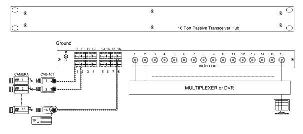
CVB-216 is a multi video transceiver designed for one compact 19" wide 1U panel. Panels can reside in the same rack as other equipment, such as switchers, multiplexers, DVR, video conferencing equipment, etc. It's perfect for larger CCTV installations and ideal for security monitoring stations.
