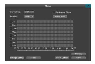
Note: If check Continuous Alarm, it will keep Alarming when Motion is detected. If not check the Continuous Alarm, the alarm only happened one time.
