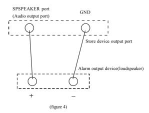
Active output alarm device has power itself, such as loudspeaker: between the cathode of Capacitor connect a wire to the AUDIO OUT; the another port of alertor connect to the GND of AUDIO OUT, as figure 4.
