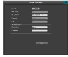
3) Add IPC one by one, Click " to add an IPC, when the status shows " , it means you can add it directly, no need to input user name or password; when the status shows ", you may need to input the input the user name and password of the IPC. As right picture:
