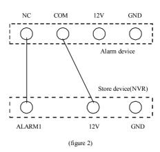
NO represent the alertor is Normally Open,in normal status, after connection the alertor as figure 1, the voltage of ALARM1 is 0V. when there is alarm triggered, it equals that the switch between the NO and COM closed, at this moment the voltage of ALARM1 is 12V, it is much more than 0.8V, therefor alarm.
